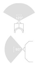
Sensors have viewing angles of 123° horizontally and 93° vertically. Lens covers to restrict the angle are available on request for specific needs.
